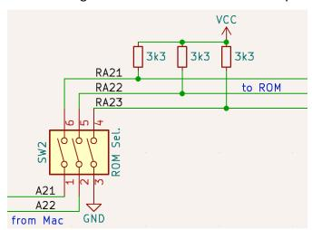
2 MB images can be flashed with the ROM Select switches in any position.
