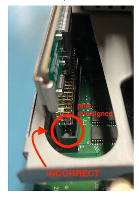
After ensuring that the card is correctly aligned with the connector pins on the Macintosh motherboard, press firmly downward to secure the RAM card in place.
