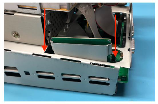
Ensure that the card is aligned correctly with the connector on the motherboard. Make sure the card is aligned correctly with the pins on the motherboard's slot such that all the pins are inserted into the card's connector. Correct and incorrect installation pictures are shown below:
