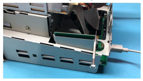
Pull the board upward using the screwdriver, alternating between the two mounting holes, until the board is loose in the socket and can removed by hand.
